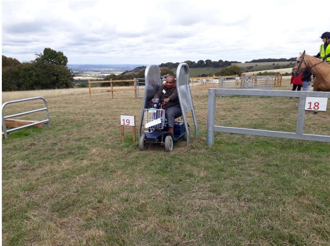
Scooter passing through a motorcycle inhibitor This model passed through easily.
